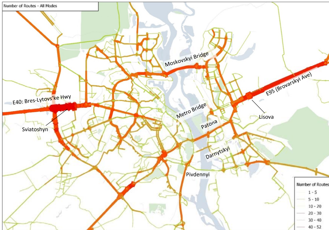
Figure 2-12: Count of all PT routes on each road segment
