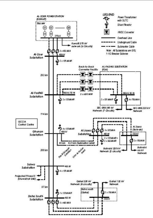
Figure 9 GCC Electricity Interconnection Phase I Diagram
