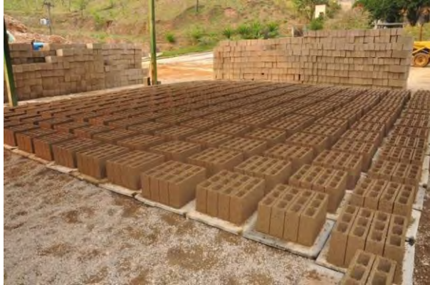
Figure 15: Bricks made from recycled construction material
