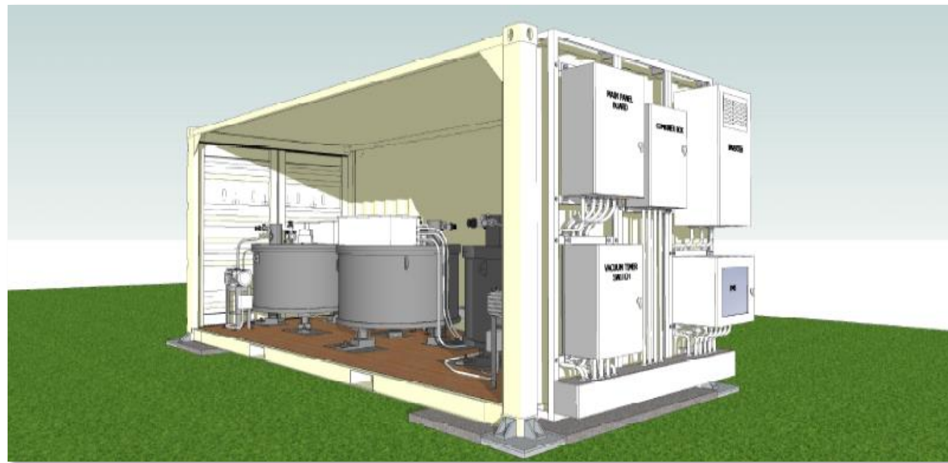
20' Containerized Solution: 3 x M32 = 24kW/96kWh
