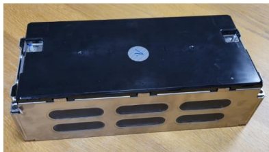
2 nd Life Electric Vehicle (EV) Battery
