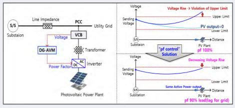
MV(13.2kV/22.9kV) interconnection configuration
