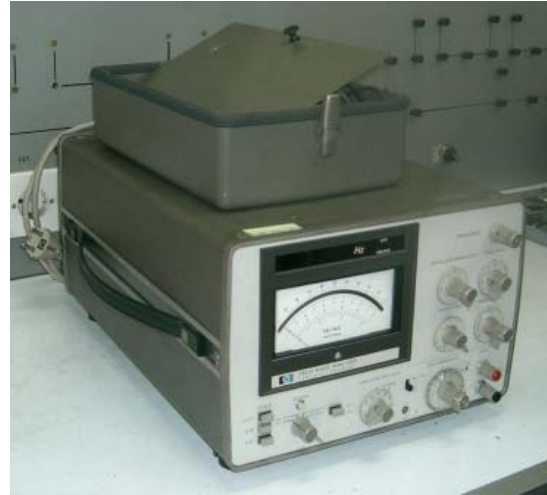
Figure 26: Power Factor and Harmonics Measuring Instruments
