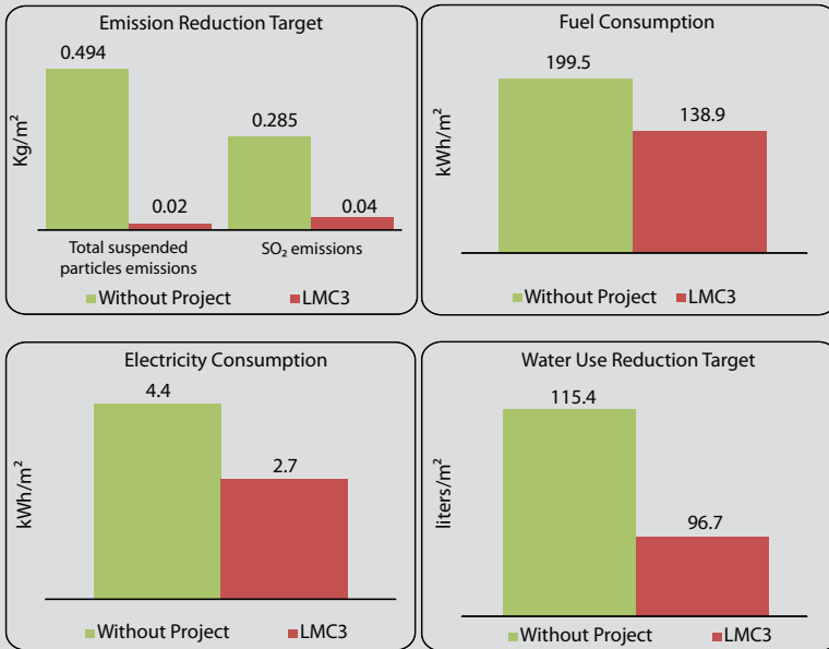
Figure B8.6.1 Project Indicators and Targets for Environmental Performance and Energy Consumption in the Liaoning Medium Cities Infrastructure Project
