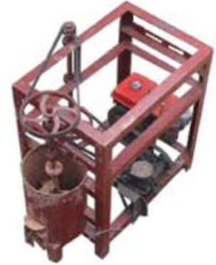
A mechanized clay mixer
