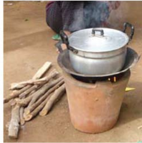
Size of cooking pot compared to size of NKS. NKS too small for the pot (L), and suitable for the pot (R). User added a rim to adapt to the small cooking pot.
