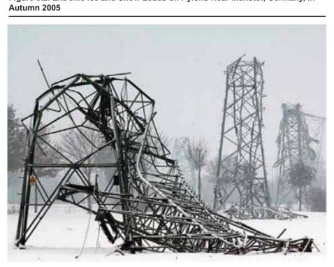
Figure 3.2. Extreme Ice and Snow Loads on Pylons Near Münster, Germany, in
