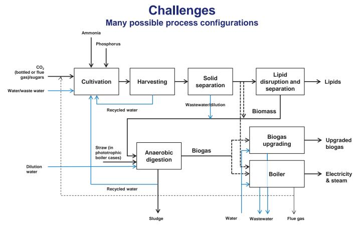
Block-flow diagram of microalgae-based energy production. Dashed lines represent alternative configurations
