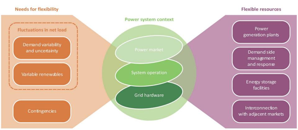
Existing and new flexibility needs can be met by a range of resources in the electricity system – facilitated by power system markets, operation and hardware.
