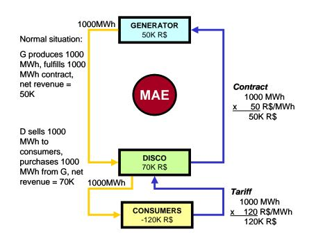
Figure 4.2: Energy Settlement Numerical Example – Before Rationing
