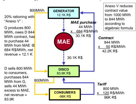
Figure 4.4: Energy Settlement Numerical Example – With Annex V
