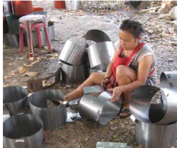
Cutting tin-coated, metal sheet wraparounds for stoves in family-owned business outside Vientiane capital
