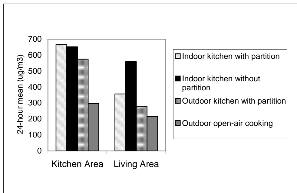
Figure 2.4. Kitchen and Living Area RSPM Concentrations for Different Kitchen Configurations in Solid-fuel Households in Rural AP
