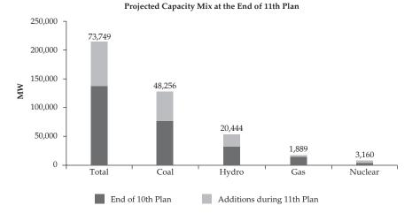
Figure A2.2: Generation Capacity Profile for India 2007 and 2007-12 Additions
