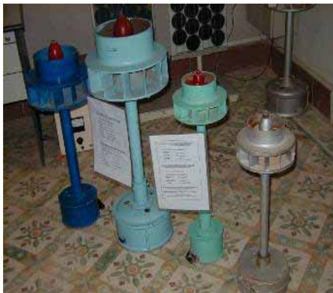
Photo A2.2: Vietnamese Family-Hydro Systems Made by RERC and Material Institute (200, 500, and 1,000 watts)
