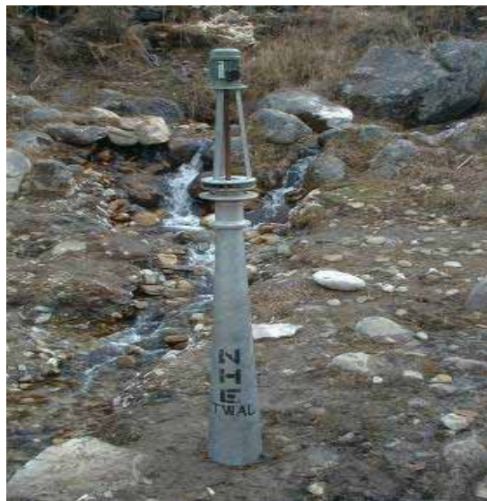
Photo A1.3: Complete PT02 Turbine Assembly
