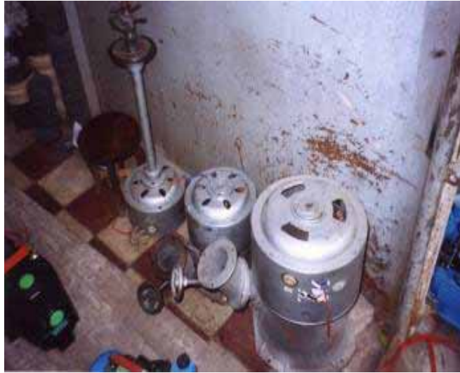
Photo A2.1: Chinese-Made Family-Hydro Systems for Sale on the Street In Hanoi (300 and 500 watts)
