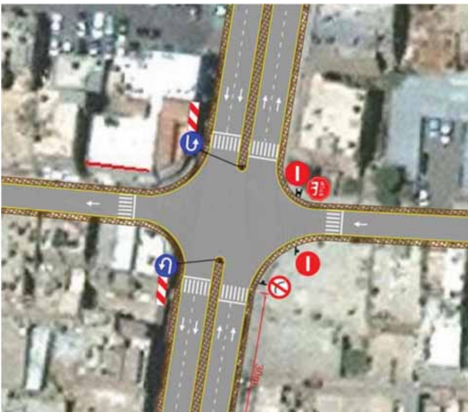
Figure L2: Example of Potential Junction Improvements
