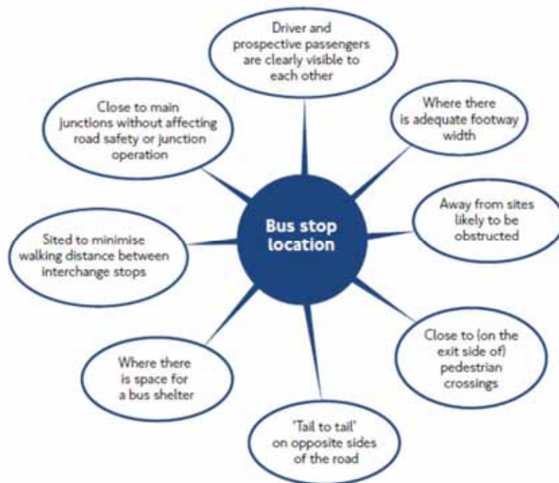
Figure H2: Considerations for Bus Stop Locations (14)
