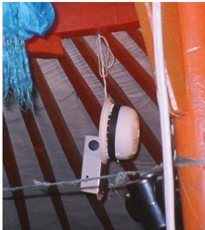
Figure 2.4: Actual Arrangement of HOBO (on Left) and UCB Monitors as Hung from Roof Rafter at Center Hub
