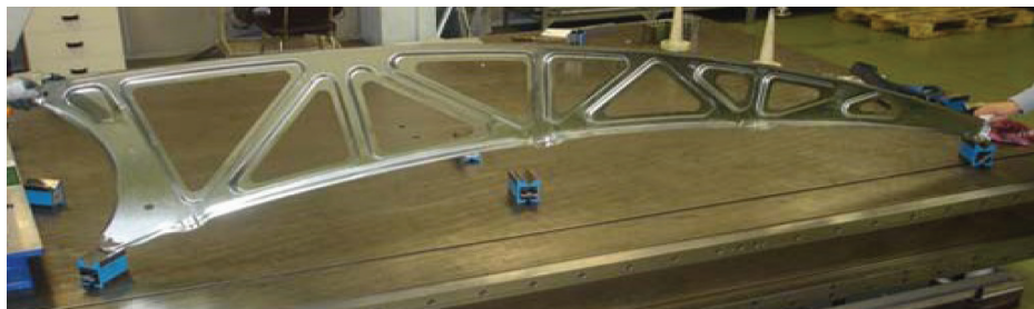
Figure 1.27 ■ Stamped Cantilever Arm by Sener; the Design was Developed to Reduce Material and Energy Demand
