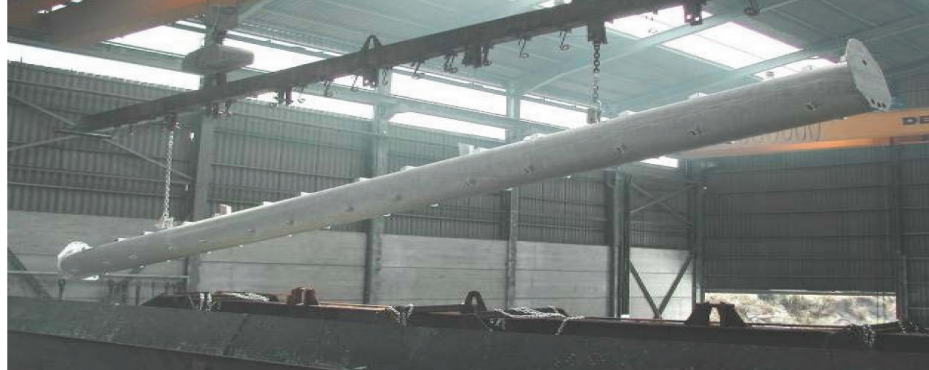
Figure 1.26 ■ Hot Dip Galvanizing of a Whole Torque Tube
