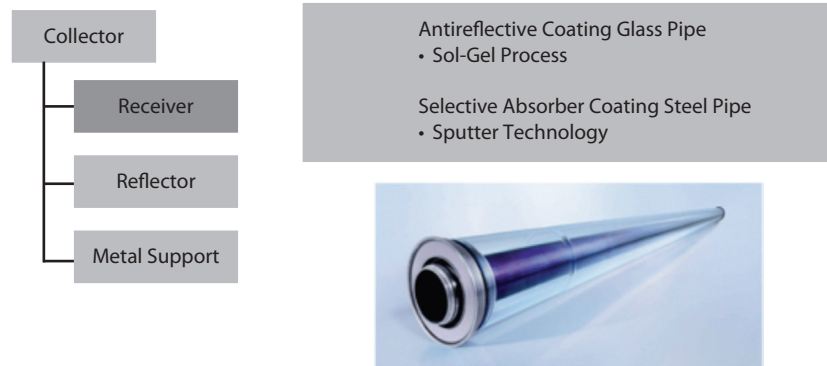
Figure 1.16 ■ Parabolic Trough Receiver PTR 70 of the Company Schott Solar
