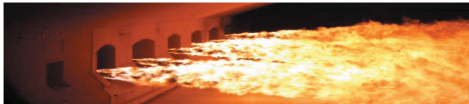
Figure 1.20 ■ Gas Heater of a Float Plant to Melt the Raw Materials Before the Float Process
