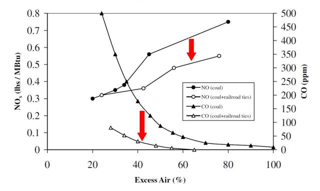
Fig. 21. Effects of co-firing 20% (mass basis) railroad ties with coal on NO<sub>x</sub> and CO emissions [76].
