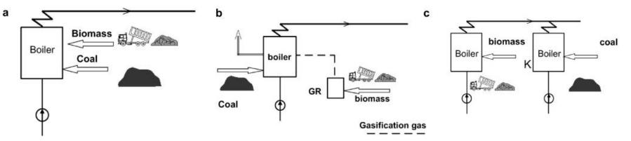
Biomass co-firing technologies. a) Direct co-firing. b) Indirect co-firing. c) Parallel co-firing from Al-Mansour and Zuwala (2010) <u>http://dx.doi.org/10.1016/j.biombioe.2010.01.004</u>
