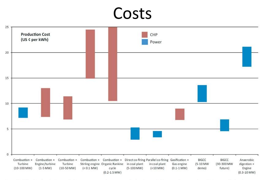
Figure 11.16 | Projected production costs for biomass to power and to CHP. Anaerobic digestion can also be operated in CHP mode; production cost will reduce by 60–80% (depending on technology and plant size) if "free" biomass feedstock is used, such as MSW, manure, or wastewater. Source: based on Bauen et al., 2009.
