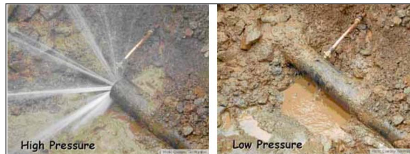
Burst water pipe at high/low pressures
