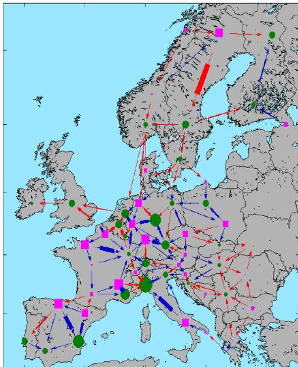
Figure 16. Annual energy flow between zones in 2020. Red: Constrained flow due to line/HVDC/NTC capacities. Blue: Non-constrained flow<sup>2</sup>. Green: Energy Deficit. Purple: Energy surplus.
